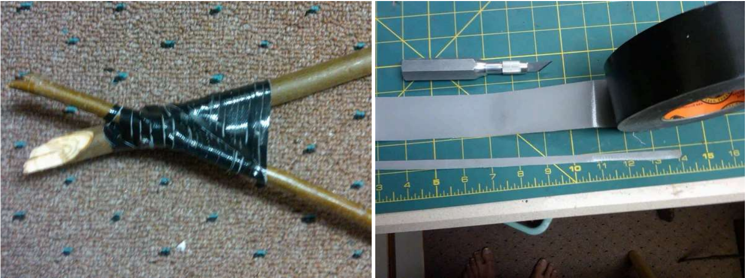
Step 6: Applying a Tape Wrap to the Back of the Snowshoes
