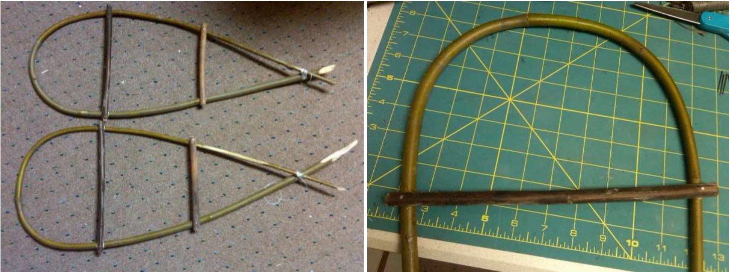
Step 5: Attaching the new cross braces to the body of the snowshoes.
