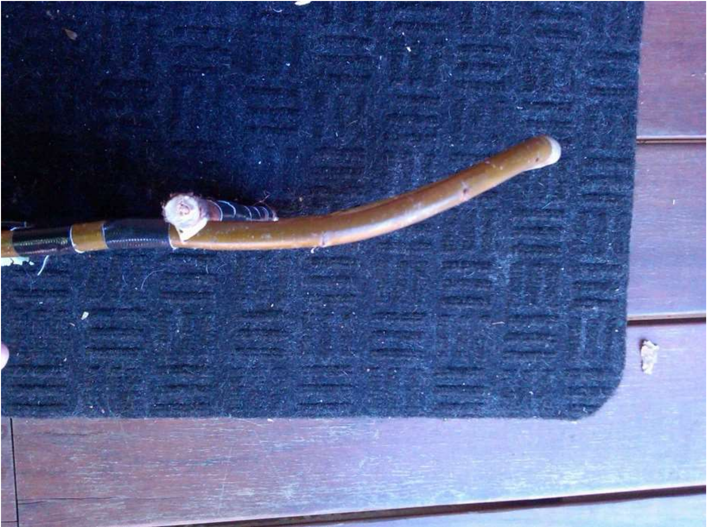
Step 11: Soaking and Bending the front of the Snowshoes
